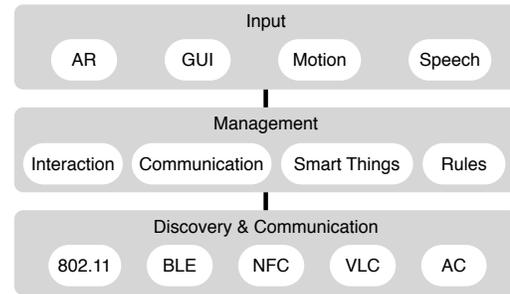
Fig. 2. Layered STIF functionality: *Discovery and communication* of and with Smart Things over a specific communication channel is matched to a specific *input* technique in the *management* layer. Rules hold a set of interaction commands to be transmitted to a set of STs over designated communication channels upon the firing of a trigger event.
