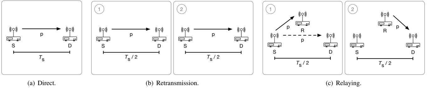
Fig. 3. Transmission options for a sending station S. In (a), S uses the whole transmission time  $T_s$  for a direct transmission of the packet  $p$  with a strong MCS to the destination D. In (b), S transmits two copies of  $p$  directly to D within  $T_s$ . In (c), S sends  $p$  via the best available relay R to D, where  $p$  might also be overheard by D when S initially transmits  $p$  to R.
