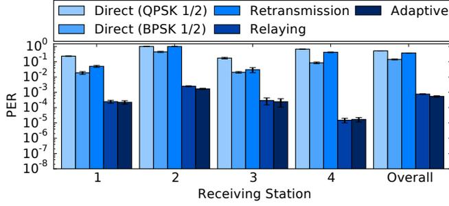
Fig. 7. Avg. PERs of different transmission options in the Static Environment. *Adaptive* represents the dynamic selection of the currently best option.
