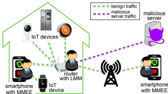
Fig. 5. Smart home with multiple IoT devices and DEMONS, i.e., an LMM deployed at the router and MMEEs deployed at smartphones. Traffic from external malicious servers is blocked as well as to/from malicious apps.
