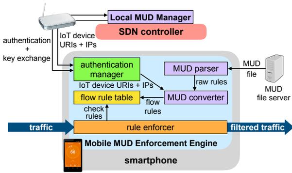
Fig. 3. MMEE architecture: the authentication manager performs authentication to the LMM, enabling local communication. The MUD parser retrieves MUD files of installed apps, extracts rules, and passes them to the MUD converter to create flow rules for filtering-based enforcement.
