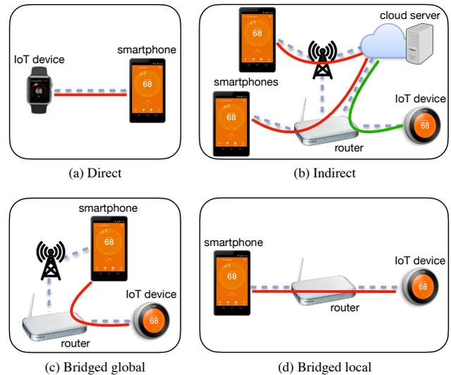
Fig. 1. Different communication scenarios between control apps (smartphones) and IoT devices. Due to dynamic IP addresses of smartphones and central enforcement, current policy-based approaches, such as MUD, only cover (b) indirect communication (green line), where the traffic flows through a cloud server. Other traffic to/from smartphones remains unfiltered (red lines).
