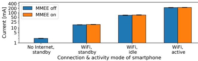
Fig. 10. Average smartphone current for different activity levels using Wi-Fi, each measured over 60 s. The first bar represents the baseline (disabled Internet, standby mode, no MMEE installed).
