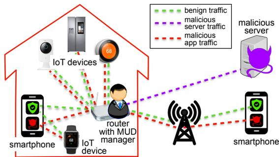
Fig. 4. Smart home with multiple IoT devices and a MUD manager [9] deployed at the router to allow traffic to/from IoT devices only according to their MUD files. While the router blocks traffic from external malicious servers, connections to smartphones are not covered including malicious apps.
