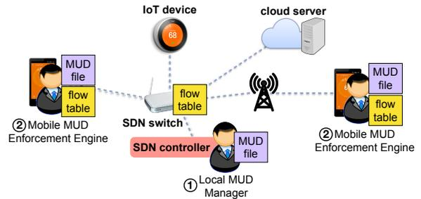
Fig. 2. DEMONS architecture [6]: ① a central LMM filters the traffic of all IoT devices in the network, enabling traffic to/from authorized smartphones and the Internet as defined in the IoT devices’ MUD files. ② MMEEs on smartphones authenticate the smartphone to the LMM and filter app traffic.
