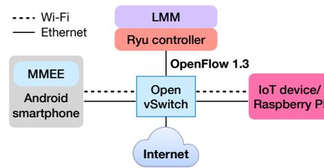
Fig. 6. Evaluation set-up of DEMONS, allowing both Ethernet and Wi-Fi connections between smartphone and IoT device / Raspberry Pi.
