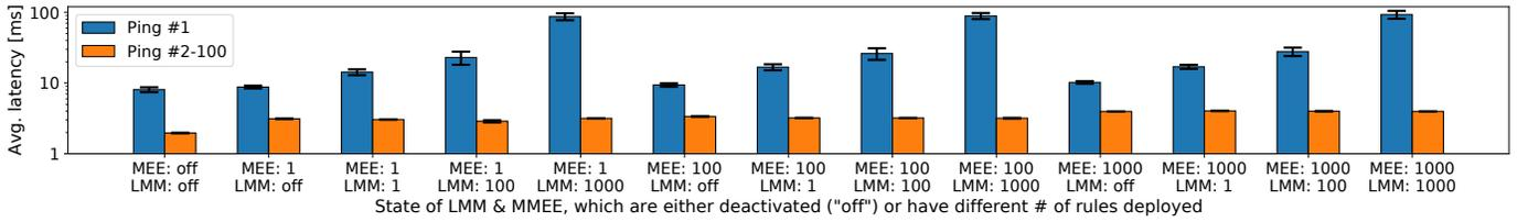
Fig. 7. Average latency with 95% confidential intervals measured for 30 runs with 100 ping messages, depending on the number of deployed rules. The first two bars represent the baseline with no traffic filtering. The latency of the first ping message is higher compared to the rest as this message is forwarded to the SDN controller before direct handling rules are installed at the switch. The latency increases with the number of rules due to higher look-up times.
