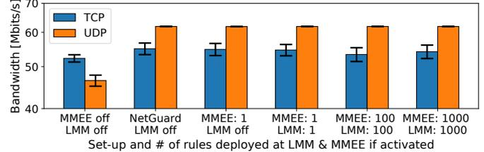
Fig. 9. Average bandwidth with 95% confidential intervals depending on the number of rules to match against and in comparison with NetGuard. The first two bars represent the baseline with no traffic filtering at all.
